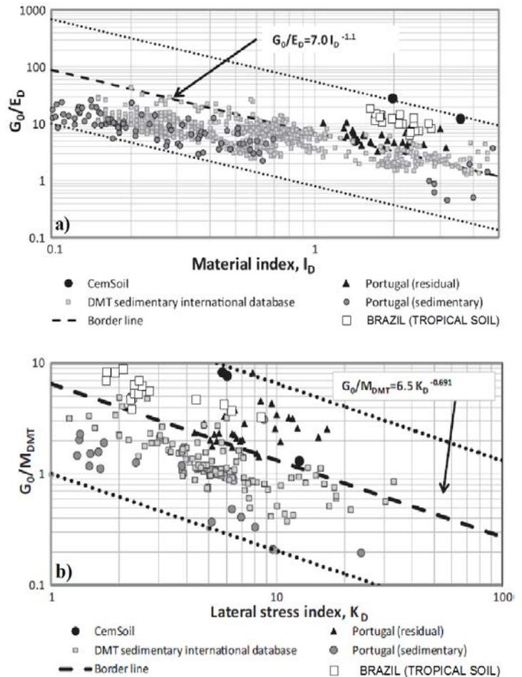
Fig. 9. SDMT tropical sandy soil data plotted on  $G_0/E_D$  vs  $I_D$  chart (Fig. 9a) and  $G_0/M_{DMT}$  vs  $K_D$  chart (Fig. 9b) (adapted from Cruz, 2010).
