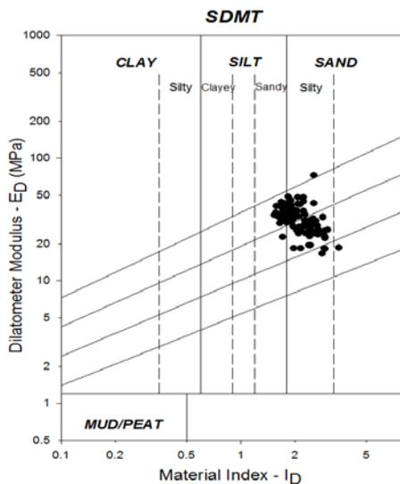
Fig. 6. Bauru site testing data position on the schematic DMT soil classification chart (Marchetti and Crapps, 1981).
