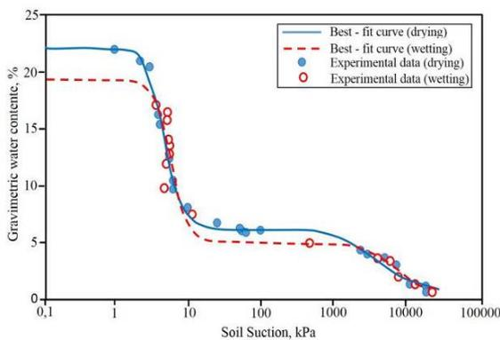
Fig. 3. Soil-water retention curve for one meter depth soil sample for the study site (Fagundes, 2014).
