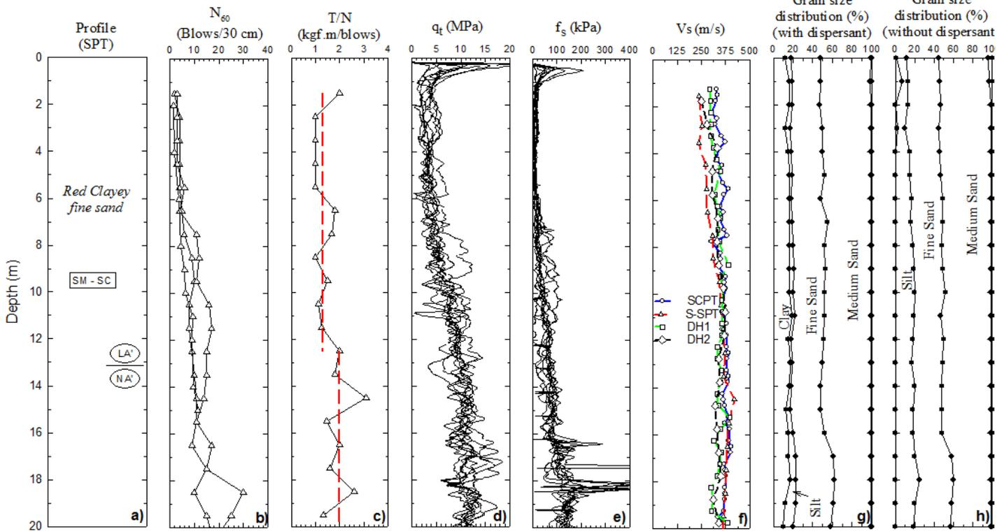
Fig. 2. Synthesis of in situ (SPT-T, CPT and Seismic) and laboratory (grain size analysis) test data for the RS2 site.
