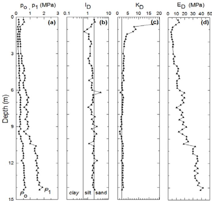
Fig. 4. DMT test data for the Bauru RS1 site.
