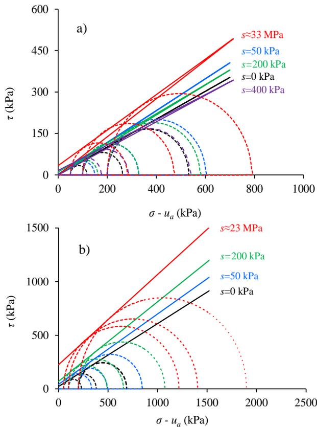
Fig. 8. Mohr circles and Coulomb failure envelopes for 1.5 m depth soil from RS2 site (a) undisturbed and (b) compacted (Fagundes and Rodrigues, 2015).
